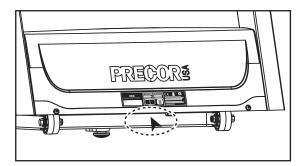
Figure 2: Power switch location
