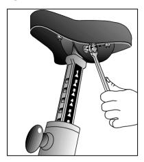
Figure 6: Loosening nut to adjust seat tilt
