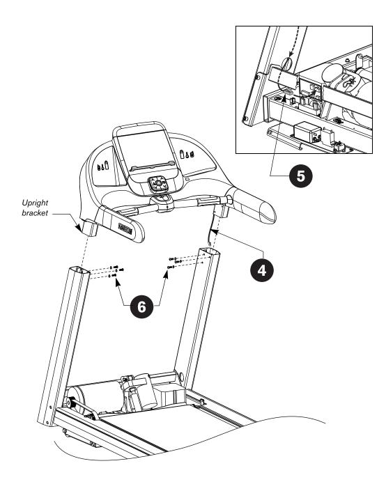
Ask your assistant to hold the display console above the upright supports while you unwrap the cable and feed the it through the right upright support.
