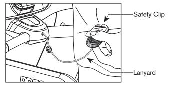
Figure 1: Attaching the safety clip
