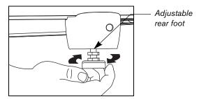
3. Retighten the lock nut and lower the treadmill to the floor.
