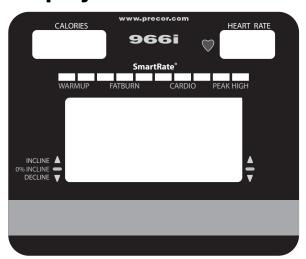
The upper display includes the CALORIES, HEART RATE, SmartRate, and a program profile display. The following descriptions explain what appears in the displays.
