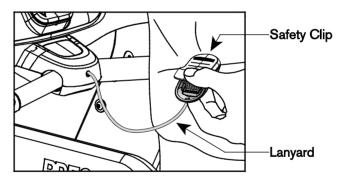
Figure 4: Attaching the safety clip
