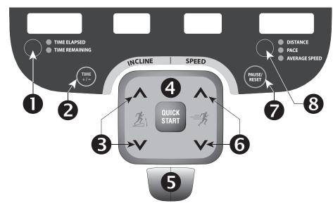
Figure 11: Lower Display keypad and the Selection keys
