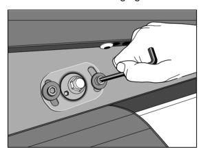
Figure 8: Loosening the two adjustment screws
