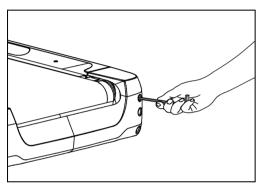
Figure 5: Location of the adjustment bolt
