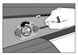
Figure 9: Realigning the center wheel
